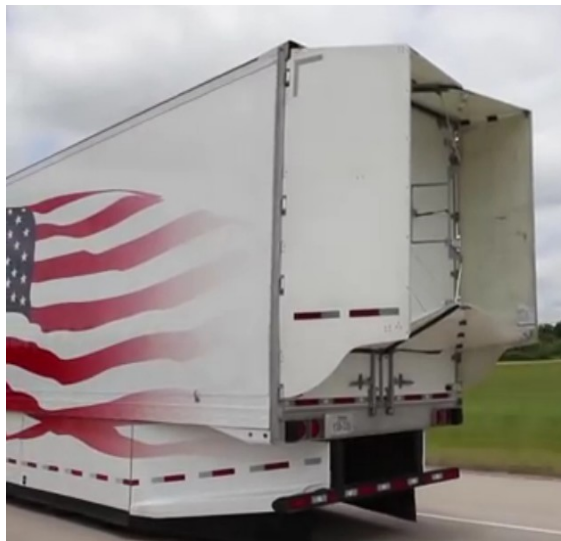
Figure 4. Super truck boat-tail flaps installation.
