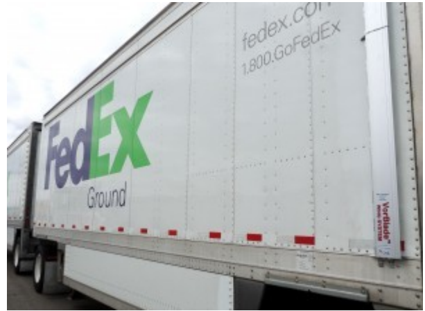
Figure 6. Vorblade trailer installation.
